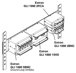
Figure 2 — Rack mounting the GLI Inhibitor
